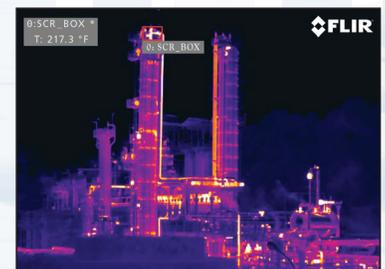
With the FC-Series R camera, you can monitor the temperature of a specific area. When the pre-set temperature has been reached or exceeded, you'll receive a notification by email, digital output or VMS alarm.
